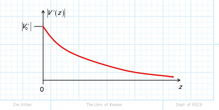
Therefore,  $\alpha$  expresses the **attenuation** of the signal due to the loss in the transmission line. The larger the value of  $\alpha$ , the greater the exponential attenuation.
